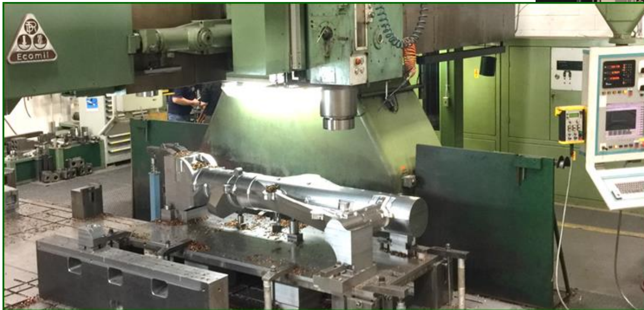
Dual spindle machine: used for E2 landing gear Machining from billet
