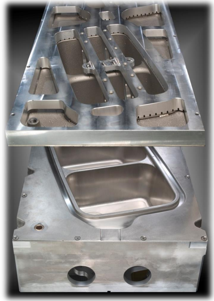
NVD Shells supported on aluminum frames
