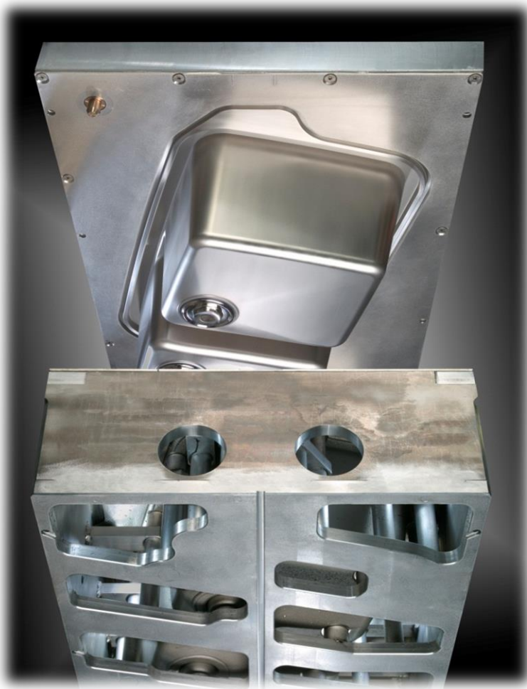
NVD Shells supported on aluminum frames
