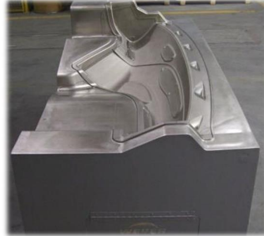
SPRAY PU MOLDS – WITH TWO COLOR SPRAY MASKS WATER HEATING or ELECTRICAL HEATING SYSTEMS
