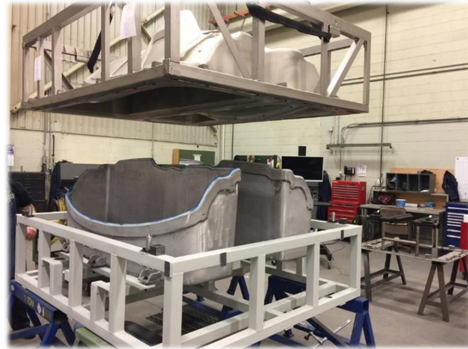
AIR HEATED NVD IP SLUSH TOOLING, TOOL CARRIER FRAME, POWDER TUBS, AND PT CARRIER FRAME ALL BUILT BY WEBER
