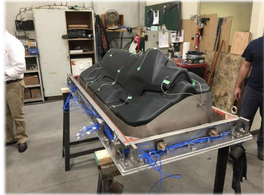
INFRA RED HEATED NVD IP SLUSH TOOLING AND MODULAR TOOL CARRIER FRAME ASSEMBLY WITH TEMPERATURE THERMOCOUPLES BUILT BY WEBER
