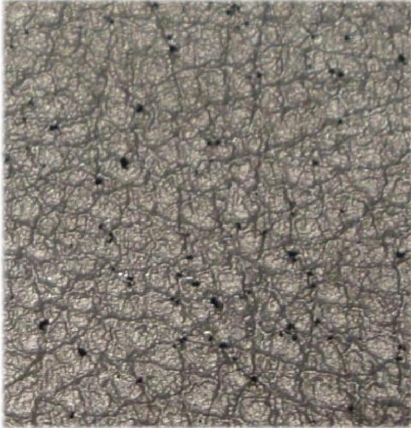
ELECTROFORM Ni SHELL VACUUM HOLE EXAMPLE
