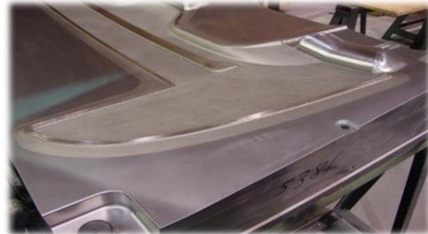
TEXTURED RIM OVERMOLDS (NICKEL SHELL MOUNTED INTO A CAVITY)
